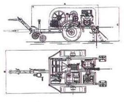
$A \times B \times C = 1,45 \times 1,20 \times 1,00 \text{ m}$ Poids (sans câble) = 300 kg
